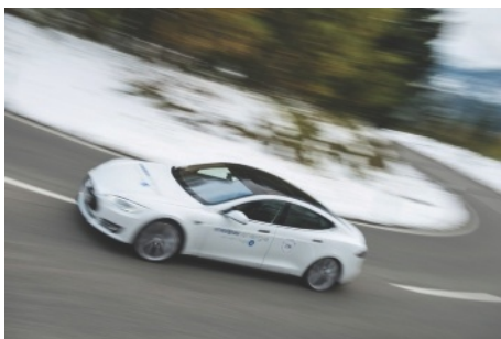
■ Figure 24.54 The Tesla Model S claims a 300 mile range from its 85kWh lithium-ion battery pack
